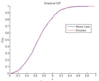
Blue line = CDF from using  $10^3$  Monte Carlo samples from the simulator Red line = CDF obtained using emulator (trained with 20 simulator runs, rational quadratic covariance function)
