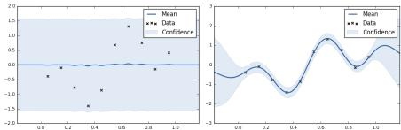
We often work around these problems by running the optimizer multiple times from random start points, using prior distributions, constraining or fixing hyper-parameters, or adding white noise.
